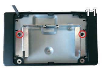
Put the screen holder on and fix only the top two screws
