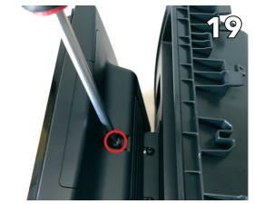
Slide the cover onto the screen and fix the screw
