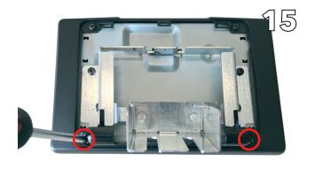
Fix the bottom cover using two screws
